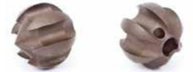
11 TULIP CUTTER The Tulip Cutter causes less damage, never gets stuck and removes debris more evenly, safely and cleanly than similar tools, such as a chain head. Ideal for removing hardened grease, lime and urine deposits and rust in pipes ranging from 50 to 125 mm.
