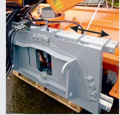
attachable frame with hydraulic lateral displacement
