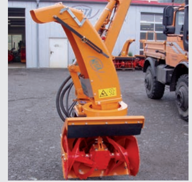
4550 / 600 AL - cantilever snow plough and thrower
