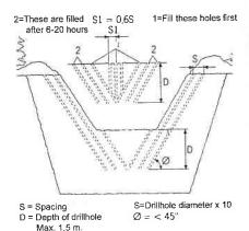
Repeat the procedure if a deeper hole is needed.
