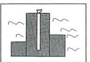
SNIGAMIT is filled in a hose of plastic film. Close both ends of the hose.
