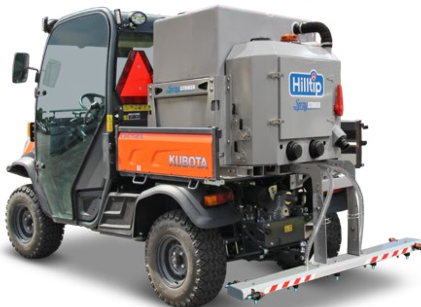
SprayStriker™ 500 on Kubota utility vehicle
