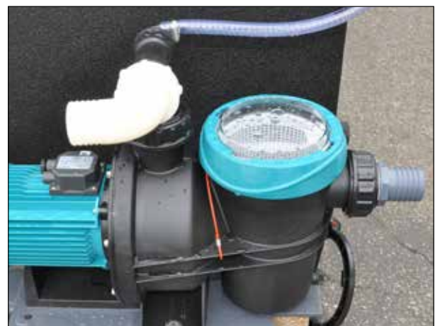
The liquid pump has a large capacity for filling spreaders or storage tanks.
