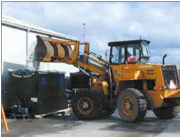
The mixing vessel is designed for easy filling using a front loader.
