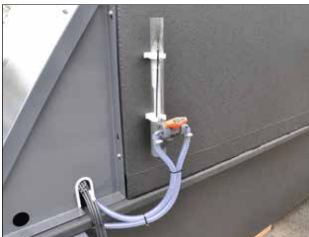
The salt solution concentration can be easily read on the hydrometer.
