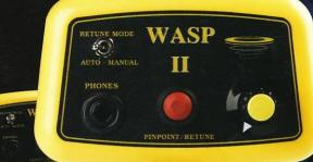
The WASP II has been designed to detect metal objects deeper while making operation of the detector extremely simple. Its self-tuning circuitry continually adjusts itself for optimum detection and is highly sensitive to all metals.
