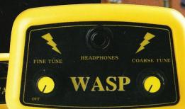
The WASP metal detector/box locator has become one of the industry's most established detectors for the location of valve covers, stop tap boxes, etc. Its simplicity of use, rugged reliability and low cost have been the reasons for its huge success.
