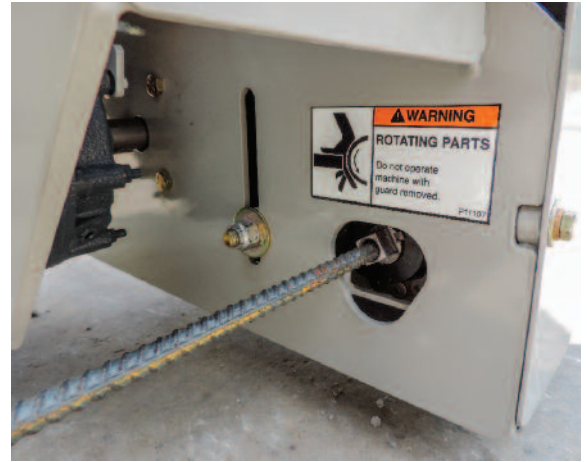
The standard hollow-shaft auger can be used for feeding longitudinal rebar through the mold.
