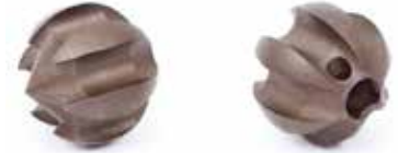
11 TULIP CUTTER The Tulip Cutter causes less damage, never gets stuck and removes debris more evenly, safely and cleanly than similar tools, such as a chain head. Ideal for removing hardened grease, lime and urine deposits and rust in pipes ranging from 50 to 125 mm.
