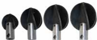
5 4 AND 6 BLADE DRILLS To mill overgrown pipes.
