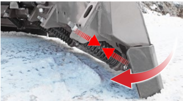
Cutting edge with trip springs
