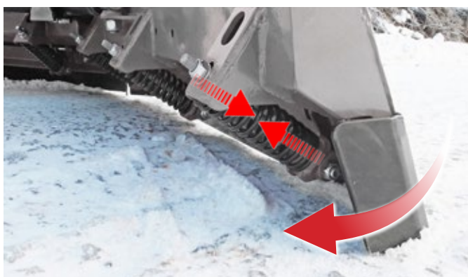
Cutting edge with trip springs
