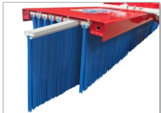
Replacing the brush rows is quick and easy
