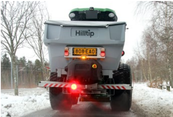
Led work light (red) and beacon light (orange)
