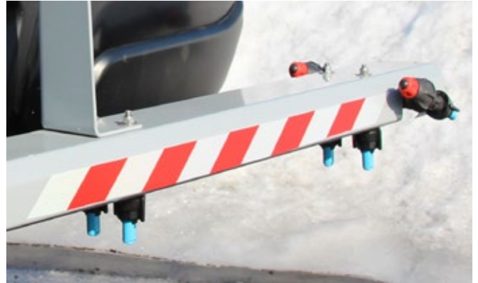
Double spray nozzles for de-icing even in high speeds.
