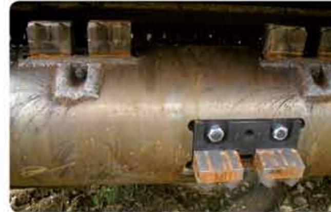
BPB-S Rotor : Standards or carbide hammers
