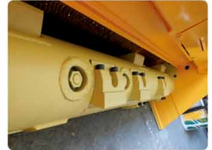
BPB Rotor : Standards hammers
