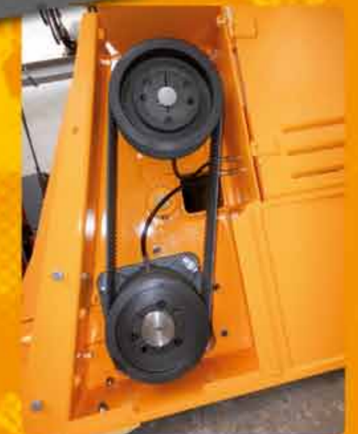
Transmission : Double drive system with special belts
