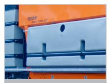
The specially developed liquid tanks ensure that there is a stable distribution of liquid contents inside the tanks. The durable liquid tanks are made from thermoplastic material, which is resistant even in extreme climatic conditions.
