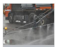
Spreading of dry matter and pre-wetted dry matter via the spreading disc. Liquid is spread via fan nozzles, which allows liquid spreading at high speeds.
