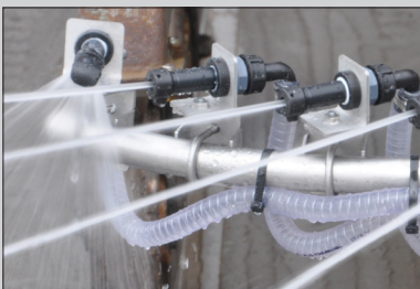
High-speed spreading using Spratronic nozzles. Spreading at all speeds of up to 90 km/h.
