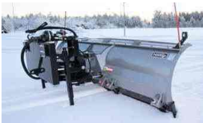
Parallel lifting device for trucks and machines with DIN plate
