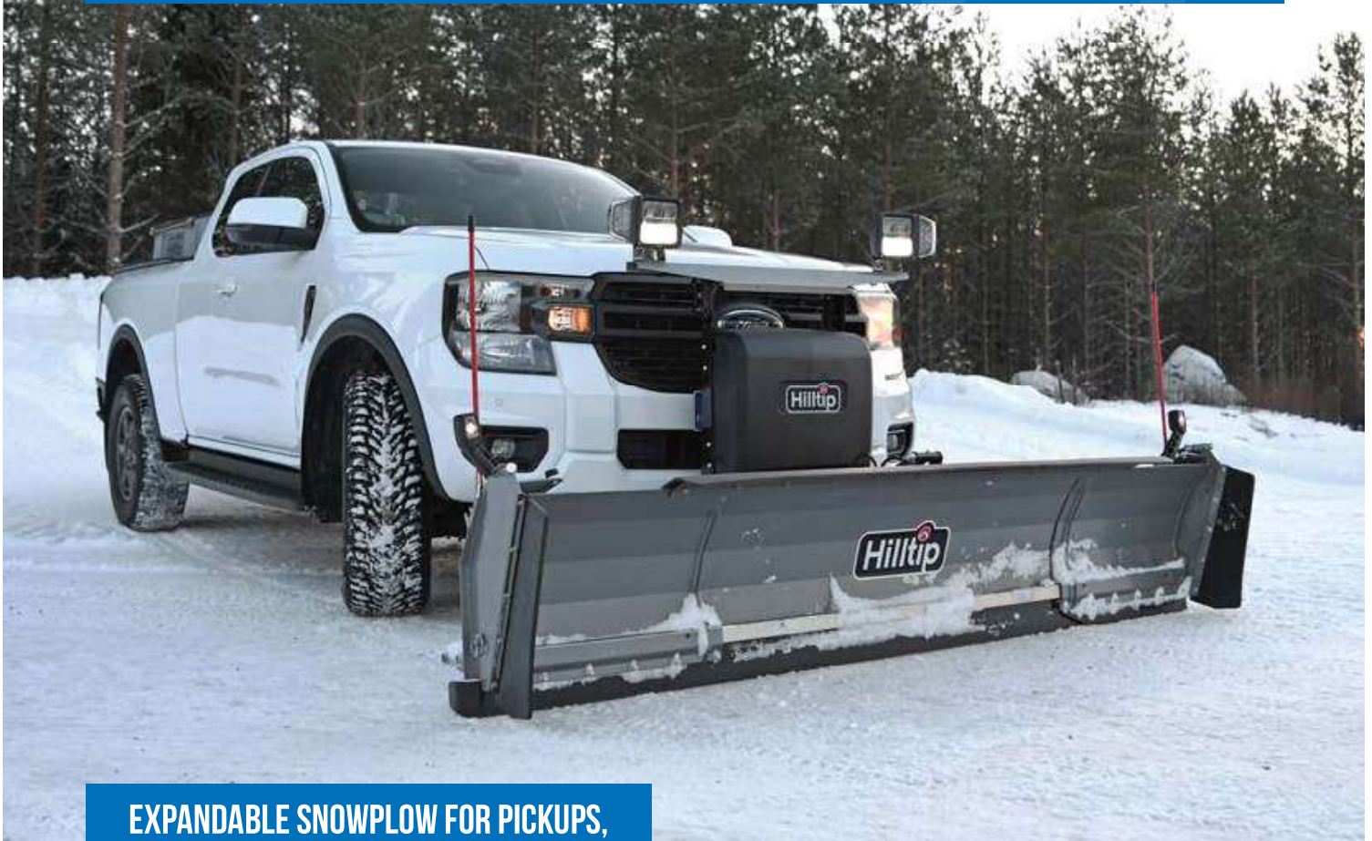
SnowStriker™ 18-26 Flex plow in extended position
