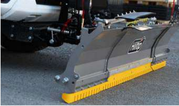
End guiding plates can be manually folded
