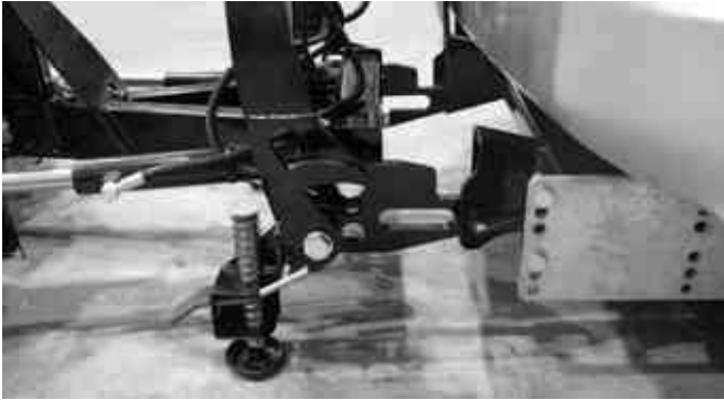
Hilltip Quick hitch - lift shoe handle to attach your plow to the vehicle
