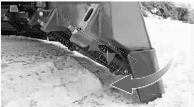
Cutting edge with trip springs
