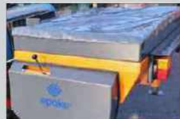
Tarpaulin to protect the spreading material when it rains or snows.
