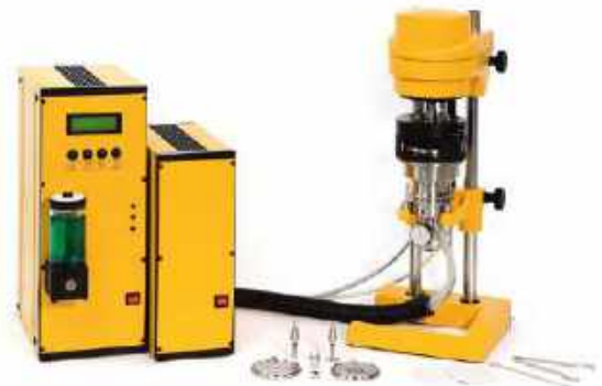
B085-08N DSR ADVANCED DYNAMIC SHEAR RHEOMETER
