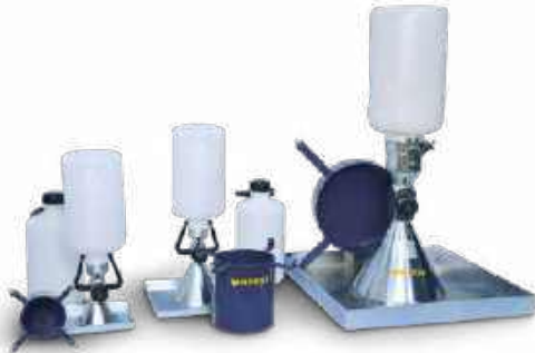
S234-01 FIELD DENSITY SAND REPLACEMENT METHOD
