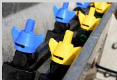
Jet nozzles with non-drip valves ensures optimum spreading profile in widths of 1–5.75 m.
