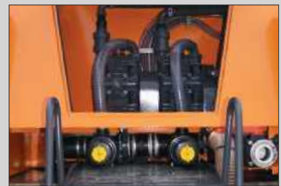
Service-friendly engine compartment with fast access to the computer unit, valves and liquid pumps.
