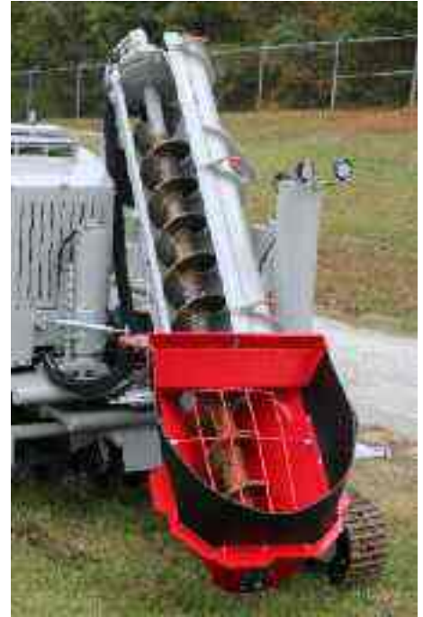
Auger Conveyor; lid opens for cleaning.
