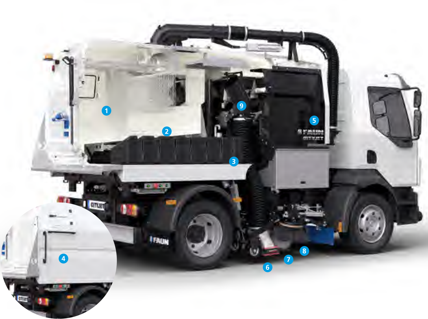
The hydraulically driven low-pressure water pump supplies the individual consumers via electric valves specially protected against calcification. The water flow delivered by the pump can be infinitely varied from inside the cab.
