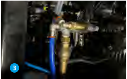
The hydraulically driven low-pressure water pump supplies the individual consumers via electric valves specially protected against calcification. The water flow delivered by the pump can be infinitely varied from inside the cab.
