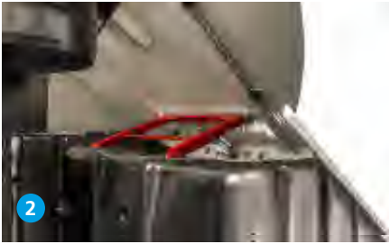
The automatic, multi-stage safety prop and check valve on the hydraulic cylinder ensures maximum safety in all situations.
