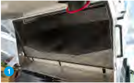
The hopper, including the tailgate, dirt collection chamber, partition walls, roof and inlet duct, is made of stainless steel.
