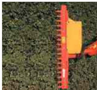
HS 16/20 Hedge-Cutter Working width: 1600/2000 mm Cutting thickness: until 45 mm Weight: approx. 120 kg/130 kg
