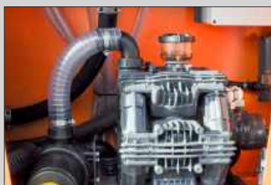
Logically designed liquid system with diaphragm pump.
