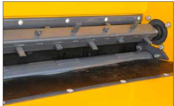
The Epoke dosing system consists of an agitator and a spring-loaded distributor roller.
