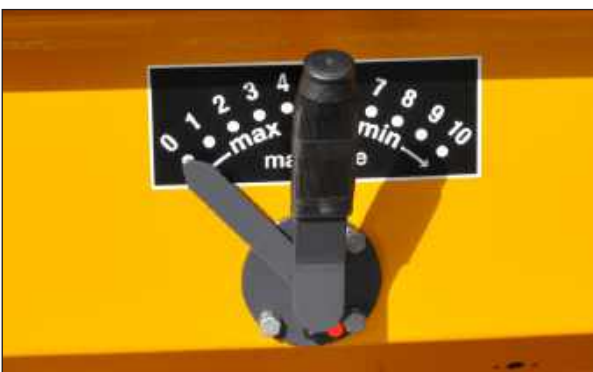
The dosing scale regulates the amount of deposited material via the connection to the spring base adjustment.
